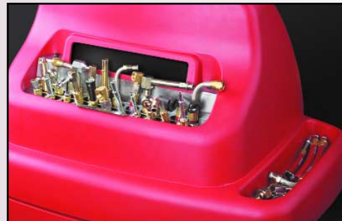
Adapters are conveniently stored in an organizer on back of machine.
